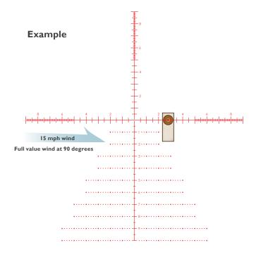
2.6 mrad correction for 15 mph wind at 700 yards. Elevation already dialed into turret.
