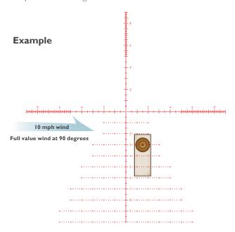
Using 3 mrad drop line at 500 yards, 1.5 mrad correction for 10 mph wind.
