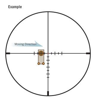
2 mrad reticle correction for a target moving 3 mph at a distance of 600 yards. Elevation already dialed into turret.
