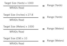
To use these formulas, it will be necessary to know the measured size of the target or a nearby object. Using either the vertical or horizontal mrad scale, place the reticle on the target of known measurement and read the number of mrads spanned. Maximum accuracy in ranging will be obtained by calculating exact mrad measurements—mrads should be estimated in 1/10s if possible.
