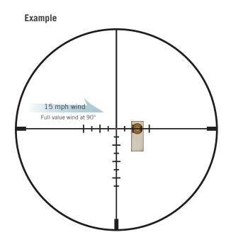
2.6 mrad reticle correction for 15 mph wind at 600 yards. Elevation is already dialed into turret.
