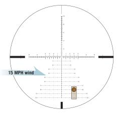
Using 8 MRAD drop line at 500 yds., 3 MRAD correction for 15 MPH wind.
