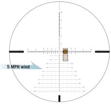
1.5 MRAD correction for 5 MPH wind at 700 yds. Elevation already dialed into turret.
