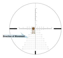
1 MRAD correction for a target moving at 3 mph at 800 yds. No wind. Total bullet time of flight from trigger pull is 1.5 seconds during which the target travels 6.6'. Elevation already dialed into turret.
