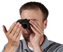
2. **Adjust the diopter:** Start by closing your left eye or covering the left objective lens with your hand. Look through your right eye and adjust the diopter ring (found on the right eyepiece) until the object is in focus. Make note of this diopter setting in case you need to set it again. From this point on, you will only need to use the center focus wheel.
