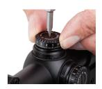
1. Remove the outer cap. While firmly holding the dial, loosen and remove center screw.
