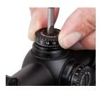
3. Install dial and reinstall and tighten center screw while firmly holding the dial...
