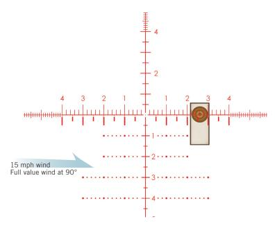
2.6 MRAD correction for 15 mph wind at 700 yards. Elevation already dialed into turret.
